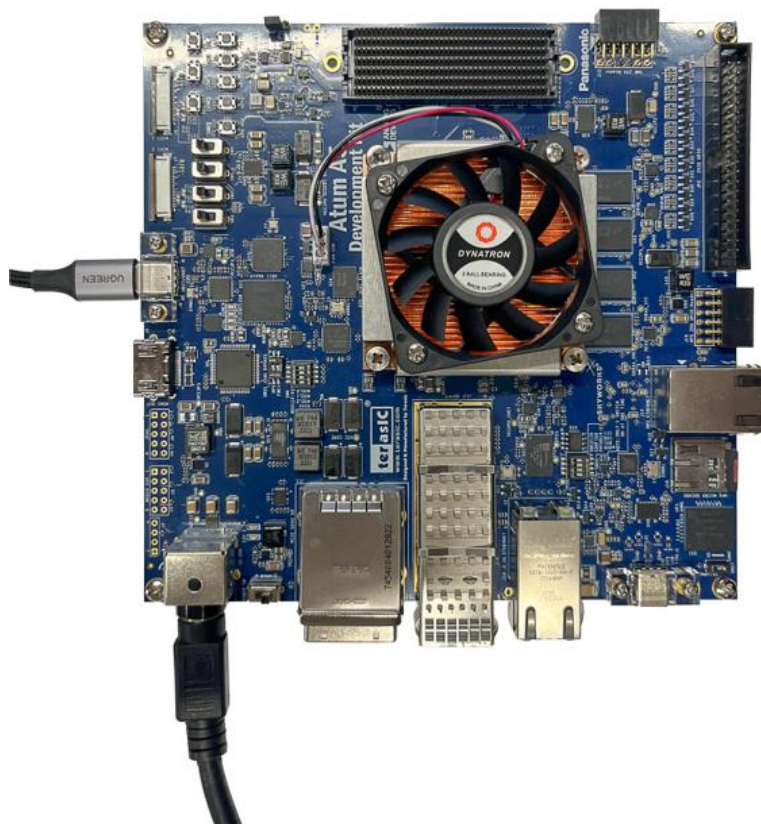
Figure 5-3 Power and USB cable connection for the board
