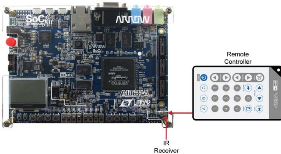
**Figure 5-14 The Setup of the IR receiver demonstration**
