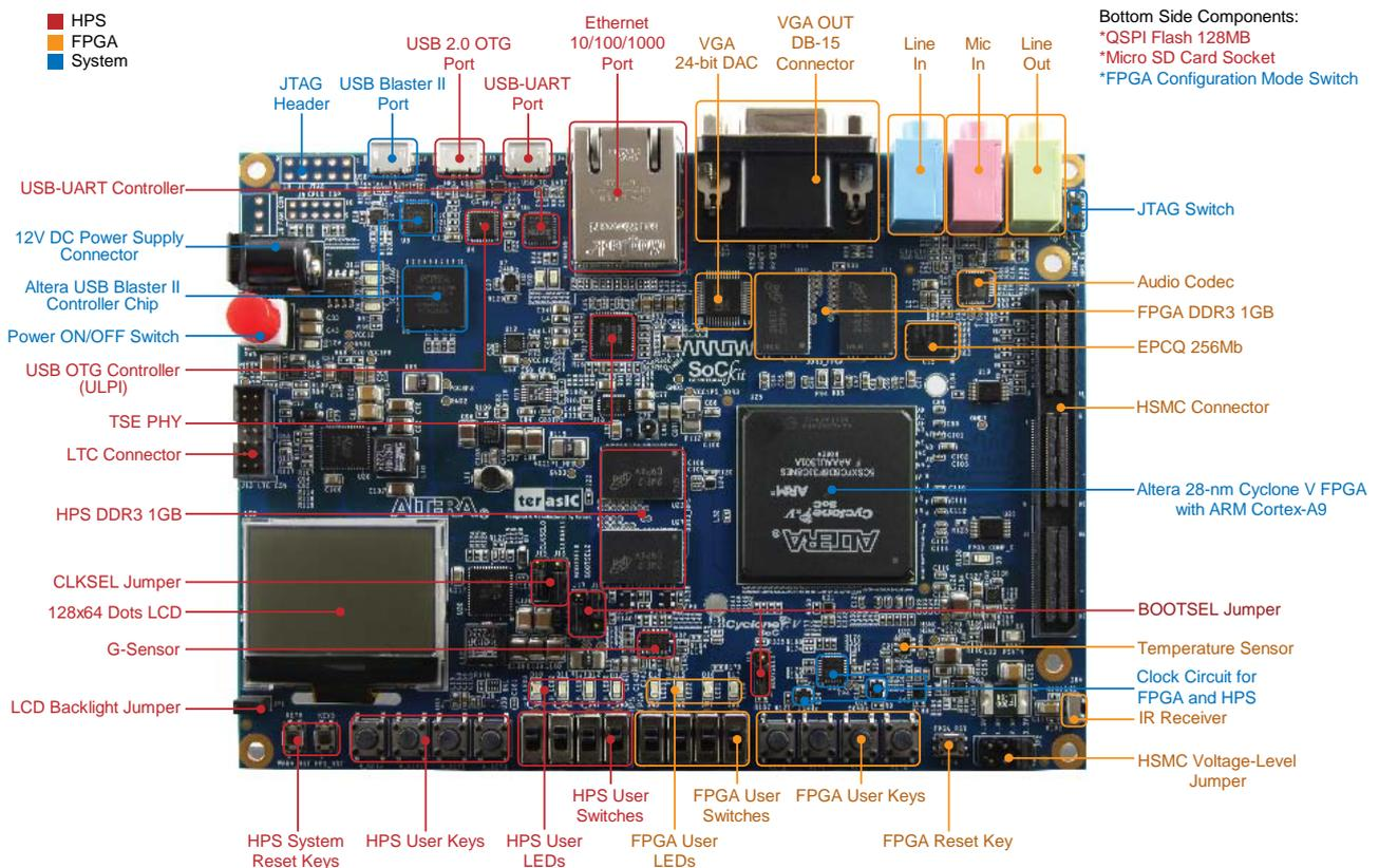
**Figure 2-1 Development Board (top view)**
