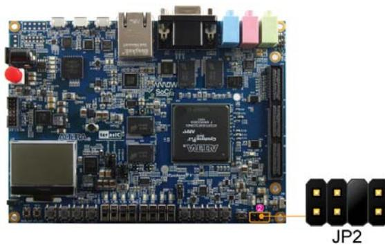
**Figure 3-6 HSMC VCCIO Voltage Level Setting Header**
