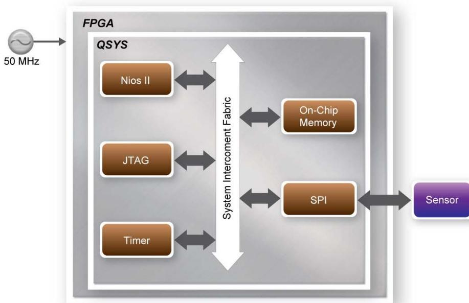
Figure 5-15 Block diagram of the Temperature Demonstration
