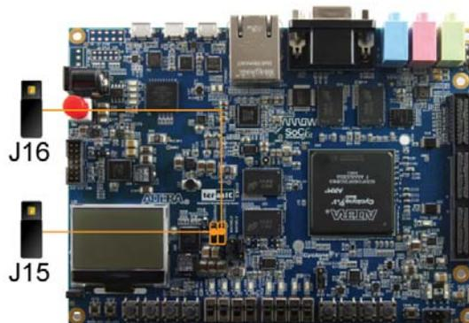
Figure 3-5 HPS CLKSEL Setting Headers
