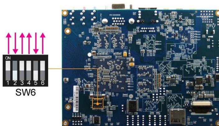
Figure 3-3 FPGA Configuration Mode Switch
