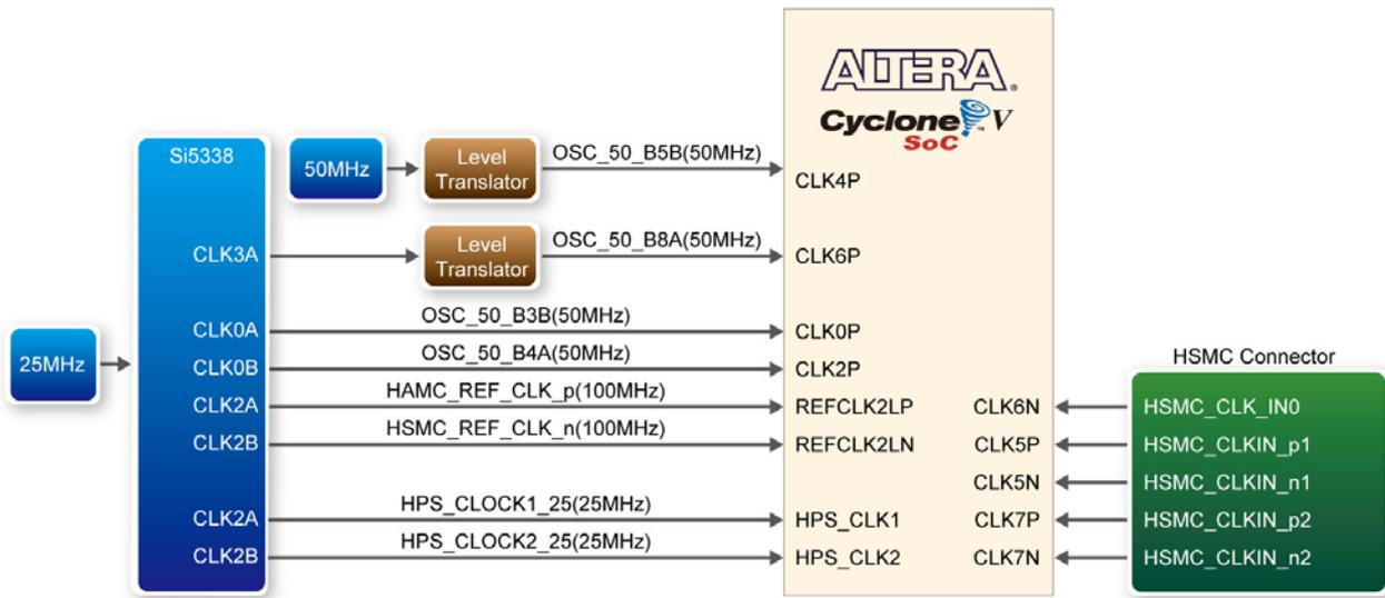
**Figure 3-10** Block diagram of the clock distribution
