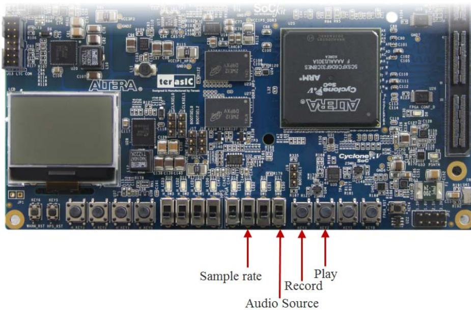
**Figure 5-1 Man-Machine Interface of Audio Recorder and Player**
