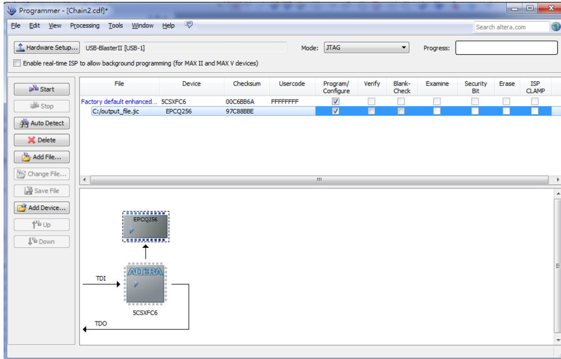
Figure 6-6. Quartus II programmer window with one JIC file
