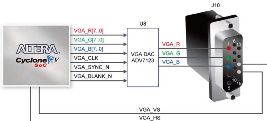
**Figure 3-17 VGA Connections between FPGA and VGA**
