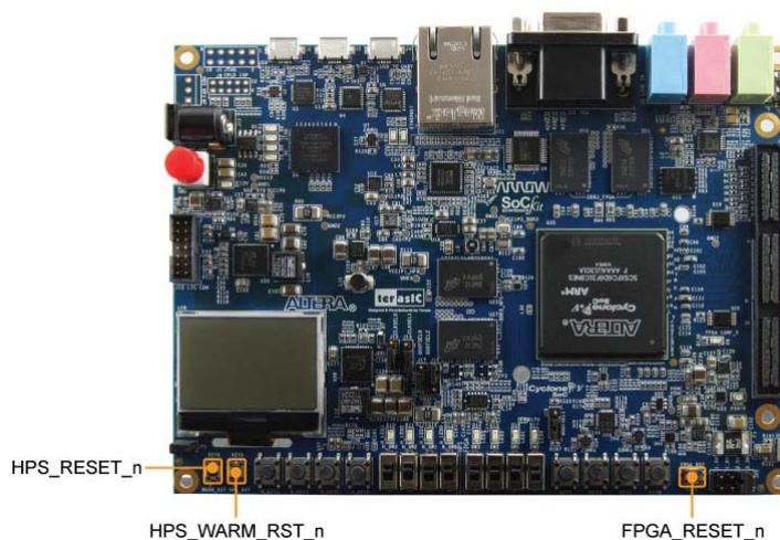
**Figure 3-7 Board Reset Elements**
