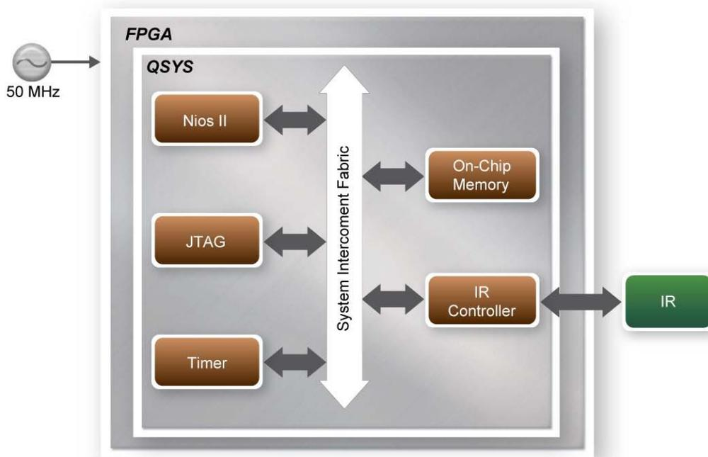
**Figure 5-9 Block Diagram of the IR Receiver Demonstration**
