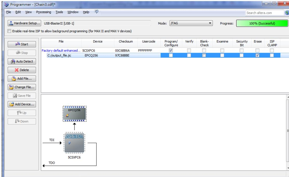
Figure 6-7 Erasing setting in Quartus II programmer window
