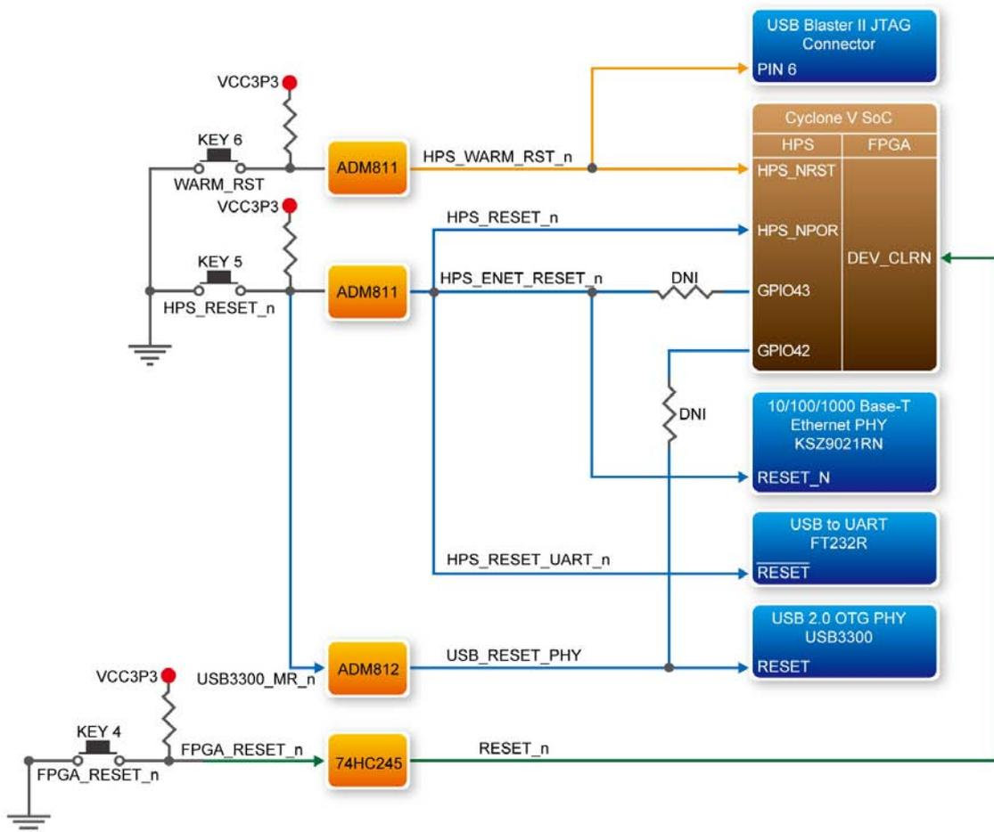
**Figure 3-8 Reset Tree on the Development Board**
