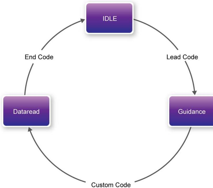
**Figure 5-12 State shift diagram of State Machine**
