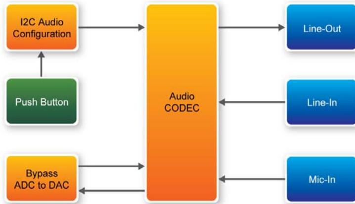
**Figure 5-3 Block diagram of the Karaoke Machine demonstration**
