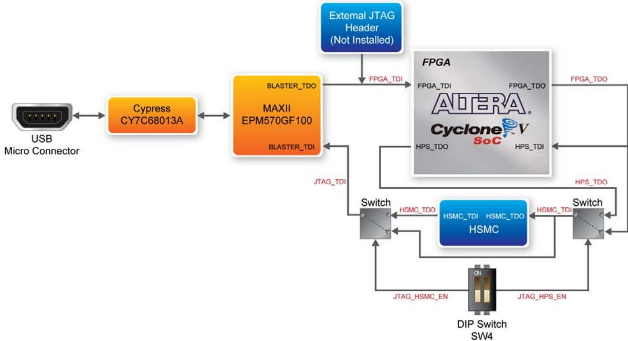
Figure 3-1 The JTAG chain on the board
