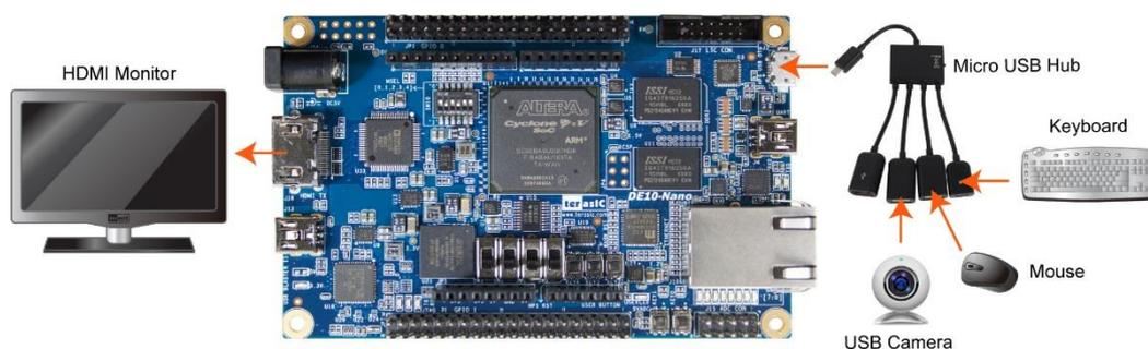
**Figure 2-1 OpenCV Setup**
