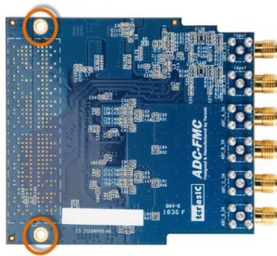
Figure 1-2 Two screw holds of the ADC-FMC
